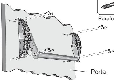
3,5) Montar as tampas sobre as bases e parafusar. Use 2 parafusos por tampa.
